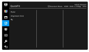
Ruler: This pattern presents physical ruler on top and left side. You can long press the Up button for 5 seconds to switch the measurements between metric and imperial.
