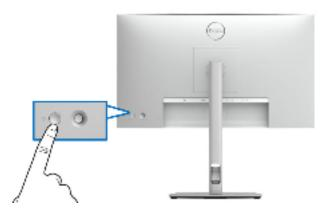
Connect/ disconnecting the DisplayPort (DisplayPort to DisplayPort) cable and Power cable
