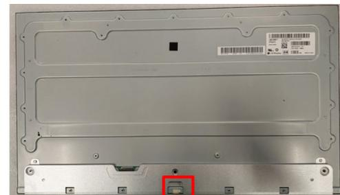
**S18** Disassemble 2 plastic BOSS from panel
