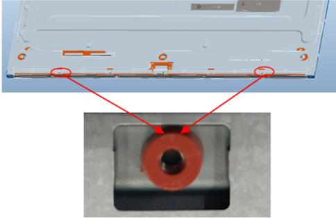
**S19** Disassemble mylar from Main SHD
