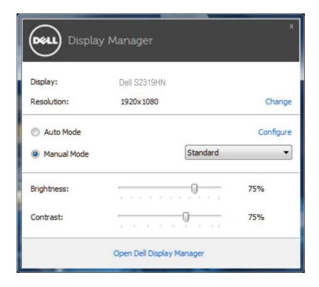
The **Quick Settings** dialog box also provides access to Dell display manager's advanced user interface, which is used to adjust basic functions, configure Auto Mode, and access other features.
