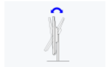
Tilt Between 5° forwards and 35° backwards
