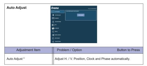
Only Analog Input. For best results, use the Auto Adjust in conjunction with the adjustment pattern. See page 27 for SCREEN ADJUSTMENTS.
