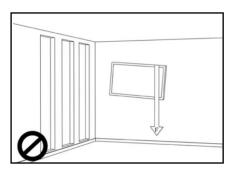
1. Do not install screens in direct sunlight, humid conditions, or high temperatures.
