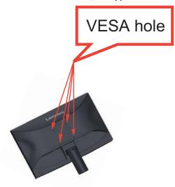
Step 5: Attach the LCD display to the wall, and follow the instructions in the wall-mounting kit.
