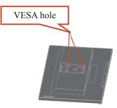
Step 5: Attach the LCD display to the wall, following the instructions in the wallmounting kit. For use only with UL/GS Listed Wall Mount Bracket with minimum weight/load: 8kg
