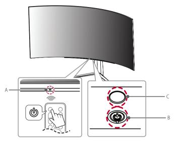
A: Remote Control Sensor B: Power Button C: Lighting
