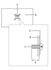
A: Wall Mount Plate B: Back of the Monitor C: Standard screw D: Max. 8 mm
