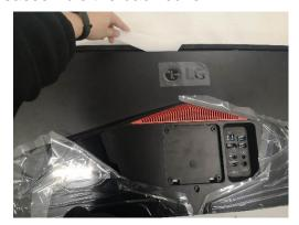
Re-overturn the set and disaaemble screw 4EA and disassemble the PCB and speaker
