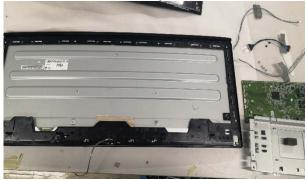
LCD module(together with their casing) is only left after all other parts like electronic units and casing have been removed.
