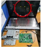
LCD module(together with their casing) is only left after all other parts like electronic units and casing have been removed.
