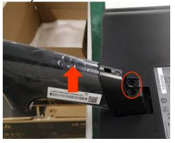
Overturn the set and disassemble the latches of three edges
