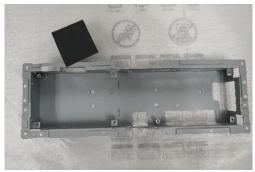
Step.9 Unscrew eleven screws and separate MID FRAME  $\operatorname{and} \operatorname{LCM}$
