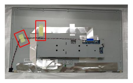
Step8. Assembly middle frame with LCM and fix screw (in red circle)
