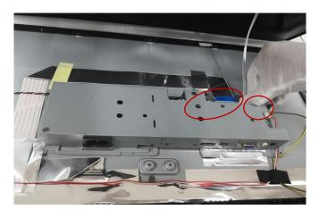
Step.5 Unscrew screws on main shielding and disassemble AL tape
