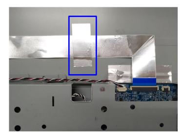
Step7. Tape AL tape to fix FFC. (Tape in red circle).
