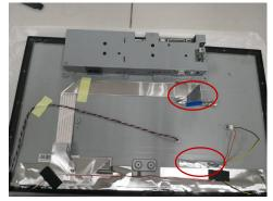
Step.6 separate SPK from MID\_FRAME and LVDS & Backlight FFC from LCM
