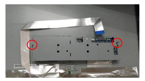
Step4. Use Al tape to fix shielding (tape in blue circle).
