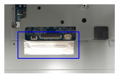
Step5. Insert 6 pin back light FFC to panel and main board, use yellow tape to fix. (Tape in red circle).
