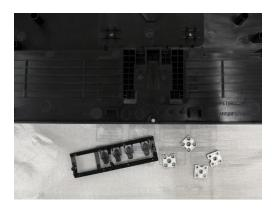
Step.13 Unscrew the screw and separate base & neck assembly
