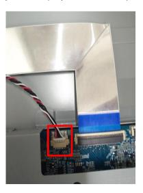
Step6. Insert 10 pin back light FFC and 30 pin LVDS FFC to main board. Use yellow tape to fix.
