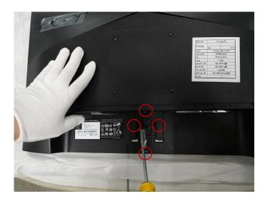
Step.3 Separate hooks between MID\_FRAME and R/C
