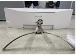
Push button and lift the stand body and remove the screw(4EA)
