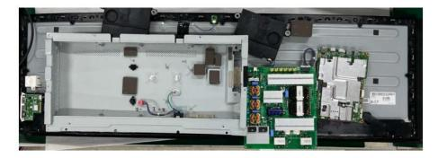
LCD module(together with their casing) is only left after all other parts like electronic units and casing have been removed.
