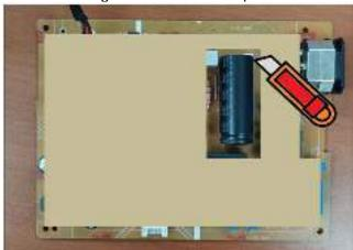
S22-2 Ensure cutting path within the glue, don't touch bulk cap. or PCB
