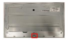
S18 Disassemble 2 plastic BOSS from panel
