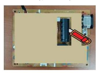
S22-3 Take out bulk cap. pin solder with soldering iron and absorber
