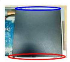
S20 Unlock 8 PCBA screws to disassemble I/F BD, SPS BD from Main SHD
