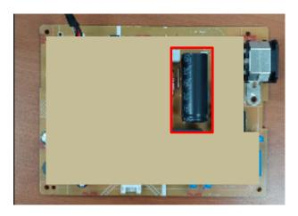
S22-1 Cut the glue between bulk cap. and PCB with a knife
