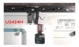
S8 Disassemble "SENSOR BD" from Middle Frame
