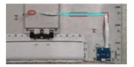
Unlock screw\*3 to disassemble CTRL BD from Rear Cover
