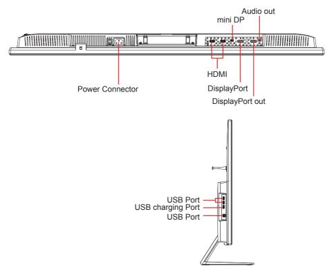
3.A. Please do not connect the DisplayPort out on the monitor to the DisplayPort or mini DP connector on the computer. DisplayPort out is used for daisy chain connection (Explained in section C)
