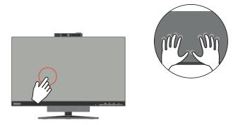
In TIO mode: You can touch screen direct to use touch function. In DP mode: You must connect external USB cable to PC then use the touch function.
