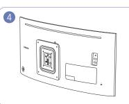
A Attach the Wall-mount bracket here
