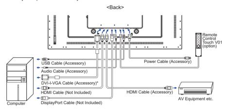
\* DVI-D cable is not supplied with the monitor. If you use low quality DVI-D cable, it may cause a result of electro-magnetic interference. Please contact the iiyama Support Centre in your country if you wish to connect the monitor via the DVI-D input.
