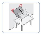
If the product is set up close to a wall and you tilt the stand to raise it up, the product may collide with the wall and become damaged. Do not raise the product with excessive force.
