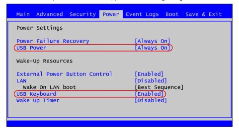
▶ In the BIOS settings on your PC, open the *Power* header where you then set *USB power* to *Always On* and *USB Keyboard* to *Enabled*.
