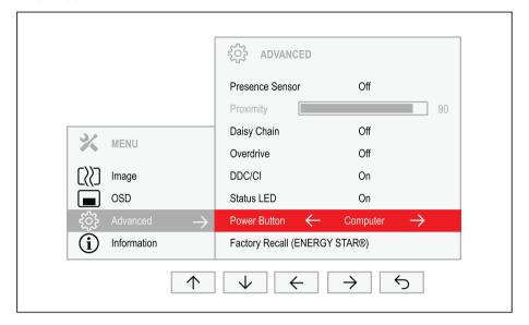
▶ In the OSD settings of your monitor, open the *Advanced* header and set the *Power Button* to *Computer*.
