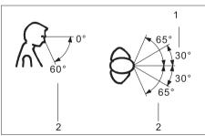
Position the monitor for optimum viewing (1). The monitor should under no circumstances fall outside the permissible viewing space (2).
