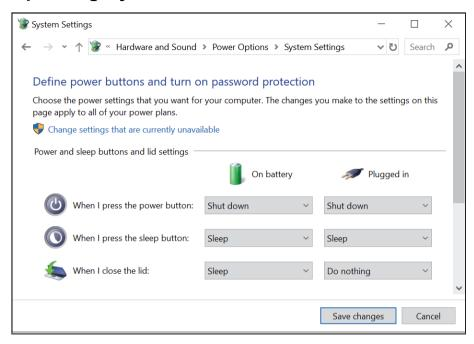
▶ In the settings of the Microsoft Windows operating system, open the *Power options - System settings* header and set the desired response characteristics of the On/Off switch.
