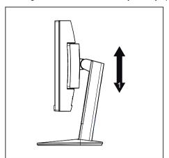
► Hold the monitor with both hands on the right and left edge of the casing and move it up or down (1).
