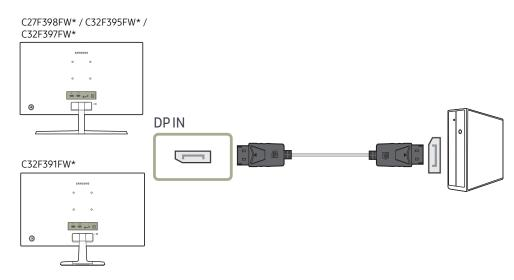
A DP cable shorter under 1.5m in length is recommended. Using a cable longer than 1.5m can affect the picture quality.
