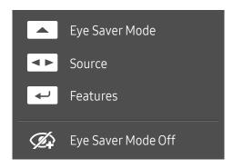
The Direct Key Guide screen shows if **Eye Saver Mode** is enabled. ( • On, • Off)
