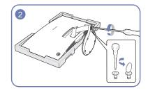
Unfasten the two screws on the stand base to remove it.
