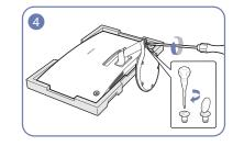
Attach the stand base to the stand neck, and then fasten the two screws on the base to tightly fix it.
