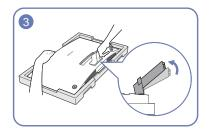
While holding the monitor, lift the stand neck in the direction of the arrow and adjust it, as shown in the image.
