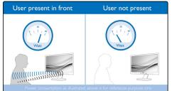
PowerSensor is a built-in 'people sensor' that transmits and receives harmless infrared signals to determine if user is present and automatically reduces monitor brightness when user steps away from the desk, cutting energy costs by up to 80 percent and prolonging monitor life
