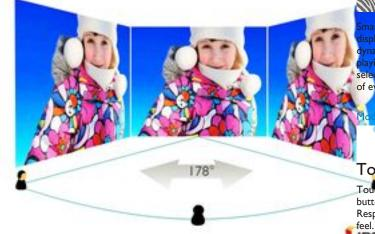
IPS-ADS displays use an advanced technology that gives you extra-wide viewing angles of 178/178 degrees, making it possible to view the display from almost any angle. Unlike standard TN panels, IPS-ADS displays give you remarkably crisp images with vivid colours, making them ideal not only for Photos, movies and web browsing, but also for professional applications that demand colour accuracy and consistent brightness at all times.
