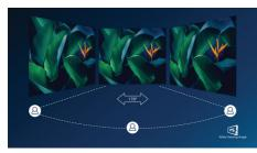
IPS displays use an advanced technology that gives you extra-wide viewing angles of 178/ 178 degrees, making it possible to view the display from almost any angle. Unlike standard TN panels, IPS displays give you remarkably crisp images with vivid colours, making them ideal not only for Photos, movies and web browsing, but also for professional applications that demand colour accuracy and consistent brightness at all times.
