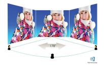
IPS displays use an advanced technology which gives you extra wide viewing angles of 178/178 degree, making it possible to view the display from almost any angle. Unlike standard TN panels, IPS displays gives you remarkably crisp images with vivid colors, making it ideal not only for Photos, movies and web browsing, but also for professional applications which demand color accuracy and consistent brightness at all times.
