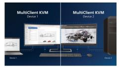
With the MultiClient Integrated KVM switch, you can control two separate PCs with one monitor-keyboard-mouse setup. A convenient button allows you to quickly switch between sources. Handy with setups that require dual PC computing power or sharing one large monitor to show two different PCs.
