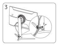
Put both cables in the cable holder on the stand (HOLDER-STAND CABLE) to organize the cables, as shown in the figure.
