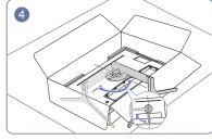
Place the stand neck of the display on the device as Turn the stand neck of the display clockwise for 90° to ensure that the stand neck of the display is put into place.
