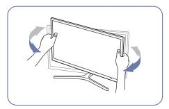
• Grasp the left and right sides of the monitor and adjust the tilt.
