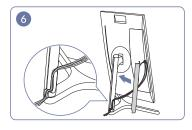
Place the corresponding cables into the standneck holder. Do not stretch the line. Three cables in one holder is recommended.
