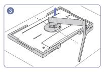
counterclockwise for 10°, lift the stand neck to detach it from the device.
