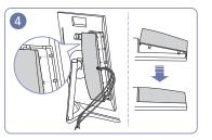
Arrange the cables through the groove on the COVER-REAR, and then attach the COVER-REAR SUB. When you attach the COVER-REAR SUB, please aim six ribs of the COVER-REAR SUB to the bottom holes of the COVER-REAR at first.
