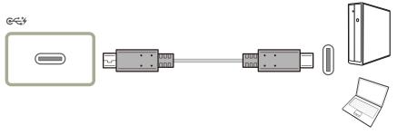
When a USB Type-C device output signals to a display, if the screen cannot display normally, please change the output mode of DP OUT (shift between USB Type-C:MST and USB Type-C:SST).
