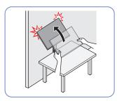
If the product is set up close to a wall and you tilt the stand to raise it up, the product may collide with the wall and become damaged. Do not raise the product with excessive force.
