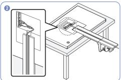
Tidy up the connected Y cable by aligning it with the stand groove, as shown in the figure.
