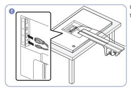
Connect the Y cables to the two ports, as shown in the figure.
