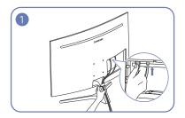
Connect cables to the appropriate ports.
