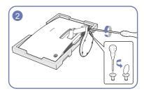
Unfasten the two screws on the stand base to remove it.
