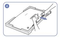
While holding the monitor, pull and remove the stand neck in the direction of the arrow, as shown in the image.
