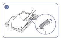
While holding the monitor, lift the stand neck in the direction of the arrow and adjust it, as shown in the image.
