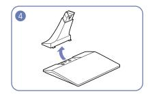
Remove the stand neck from the stand base by pulling it in the direction of the arrow as shown in the figure.
