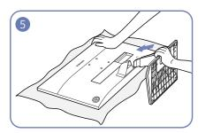
Insert the stand head into the connection hole in the direction, as shown in the figure.
