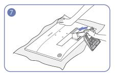
Push the assembled stand into the main body in the direction of the arrow, as shown in the figure.
