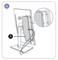
Arrange the cables through the groove on the back of the product, and then attach the COVER-REAR SUB (A). When you attach the COVER-REAR SUB (A), please aim six ribs of the COVER-REAR SUB (A) to the back of the product at first.
