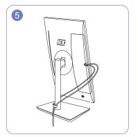
Arrange each of the two cables through either side of the HOLDER-STAND CABLE, as shown in the figure.
