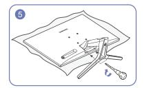
Fasten the screws at the bottom of the stand neck.
