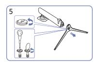
Relaxation fasten the connecting screw at the bottom of the stand base.
